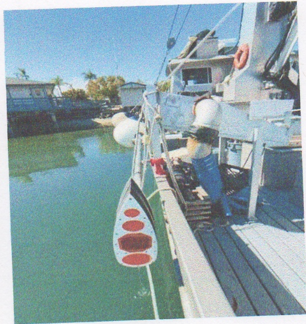
Figure F1. A four-frequency scientific echosounder system installed aboard F/V Long Beach Carnage , consisting of four Simrad EK60 General Purpose Transceivers (GPTs), a system control and data logging laptop computer, an Ethernet switch, and a GPS receiver, (left); and a retractable multi-transducer array (MTA-4) mounted on the port-side (right).
